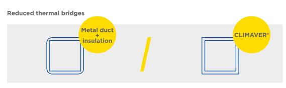
Reduced thickness of insulation at the edges
