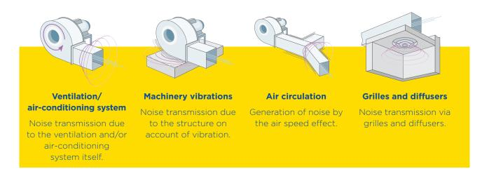
This phenomenon is particularly noticeable if the internal surface of the ducts is made of a material that easily reflects sound, e.g. metal.
