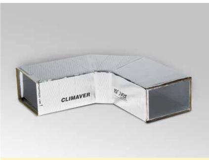
TRAIN CLIMAVER® is a high density rigid mineral wool slab with shiplaps, faced externally with a reinforced kraft aluminium foil and internally with a black glass fabric of high tensile strength and resistance for cleaning methods according to UNE 100012.
