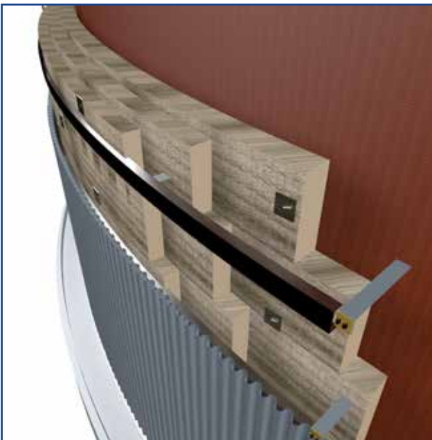
Figure 22. STORAGE TANK DETAIL 1 (Wired Mats)
