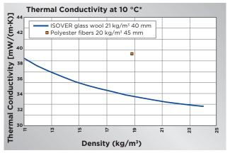
\*Thermal Conductivity at 10°C according to EN 12667
