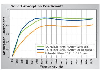
\*Sound Absorption Coefficient according to ISO 10534-2
