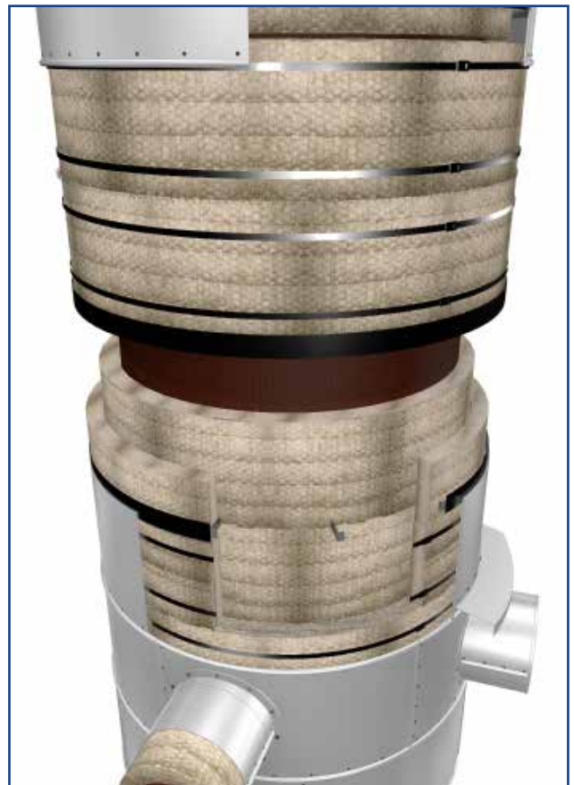
Figure 17. VERTICAL VESSEL DETAIL 2
