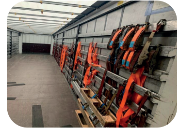
2 Lorries without racks, with gaps of at least six slats between stakes and fitted with straps
