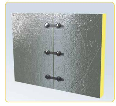
The different **U SeaProtect**<sup>®</sup> **Slab 66** panels are interconnected by steel connecting bridges (maximum spacing approximately 200 mm). Connecting bridges are used for both vertical and horizontal joints and consist of steel pins, washers and perforated steel strips on both sides of the extension.
