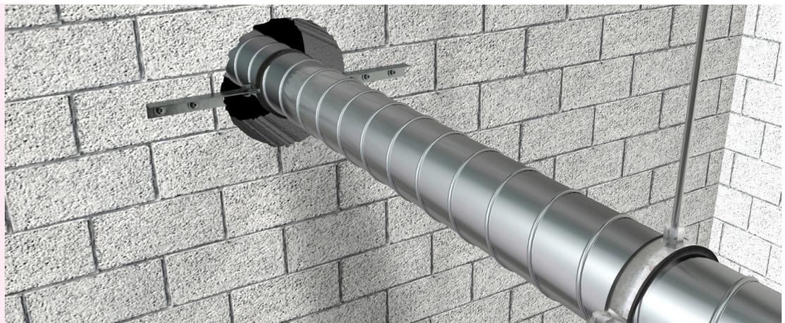
Fix steel L-profiles (dimensions 30 x 30 x 3 mm) to the wall on each side of the penetration or to the top side of the floor penetration. Secure the duct with duct hanger clamps (30 x 3 mm), encircling and attached to the duct.
