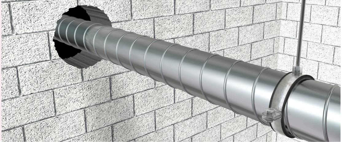
The duct is placed in the centre of the opening in the construction. The opening must be dimensioned so that when the insulation is added, the gap between the insulation and the support construction is < 25 mm. For horizontal ducts, use steel drop rods for the hangers. The tension in the rods should not exceed 9 N/mm<sup>2</sup>. The maximum distance between the hangers should not exceed 1525 mm. For vertical ducts, the distance between supporting constructions should not exceed 5 m.
