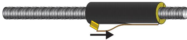
**STEP 3:** SEAL THE SEAMS BETWEEN THE SECTIONS WITH PROTECT BLACK TAPE.
