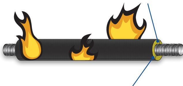
80 MM INSULATION THICKNESS => **EI60**
