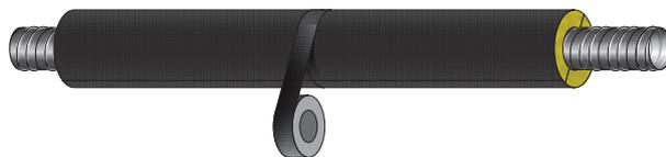
**STEP 4:** SECURE THE INSTALLATION WITH 0,7 MM STEEL WIRE IN MAX. 250 MM INTERVALS.
