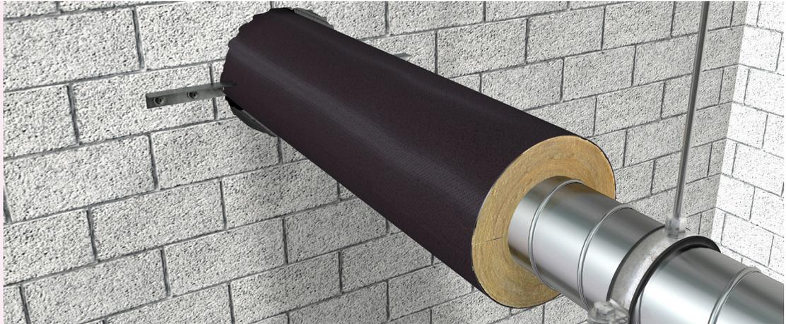
Install the **U PROTECT® VENT SECTION** around the duct. Make a small cut and push it against the L-profile into the opening. The insulation goes through the penetration. Fill the remaining gap fully with standard gypsum plaster. Note that the gap for floors can be also filled with mortar.
