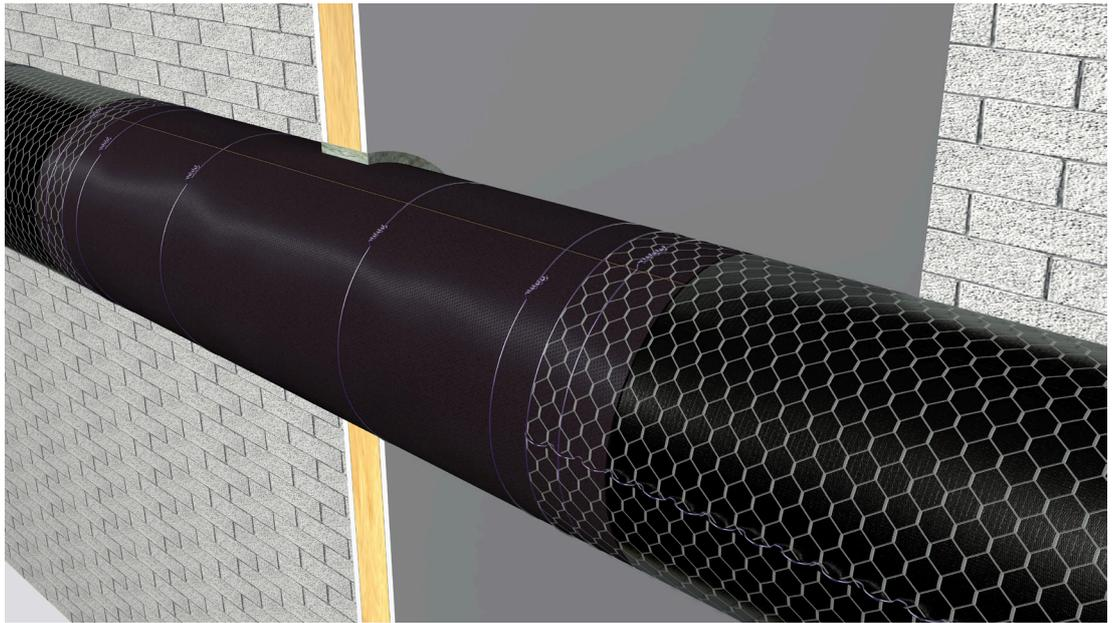
The wired net overlap should be a minimum of 100 mm in order to guarantee the perfect connection of the **U PROTECT® VENT SECTION** with the **U PROTECT® WIRED MAT**.
