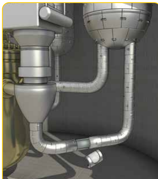
Insulation cassettes on coolant pipes
