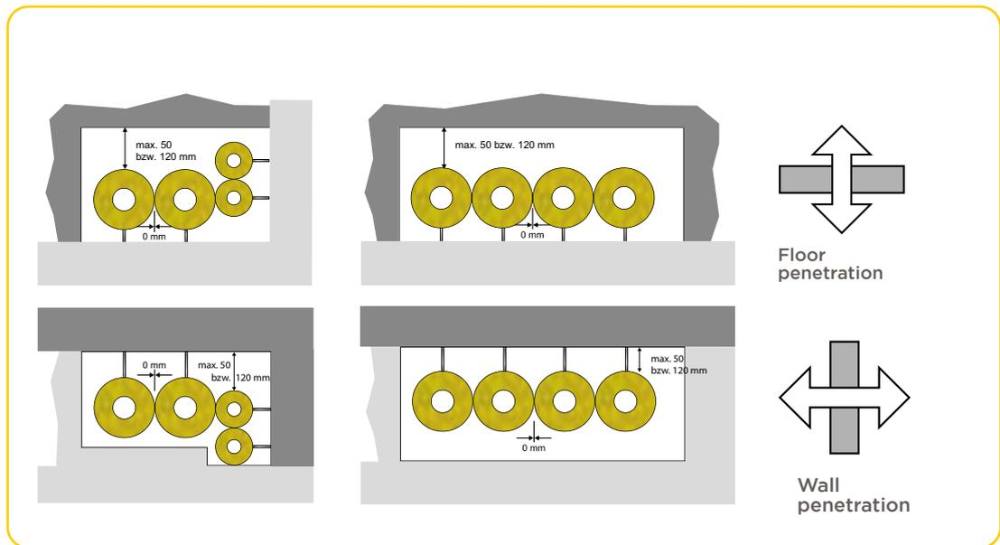
**U PROTECT® PIPE SECTIONS** can be safely installed with zero clearance, meaning that the pipe insulation of neighbouring pipes may come into contact and may also touch floor and wall openings. Various configurations are possible.
