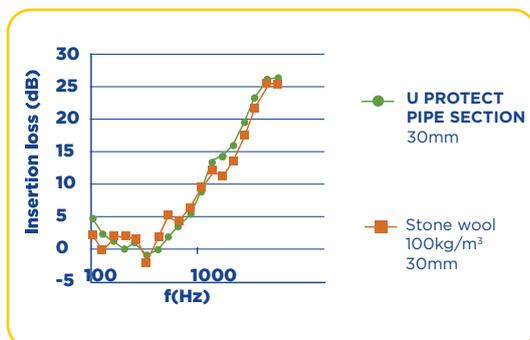
A unique value (expressed in dBA) is used to describe the weighted acoustic improvement over the whole range of frequencies measured, taking into account the non-linear sensitivity of human hearing. **U PROTECT® PIPE SECTIONS** offer a global improvement of 14 dB(A).
