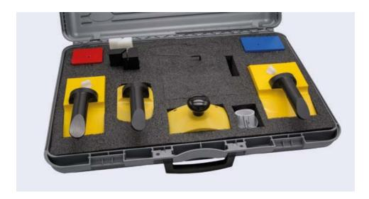
Specific cutting tools for making 40 mm and 25 mm ducts (complete CLIMAVER® range).
