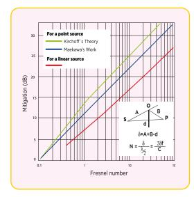
The graph shows that the sound reduction offered by the barriers depends on the dimensionless number N, which reflects the difference in path that the sound should take between the emitter (E) and the receiver (R), as well as the location of barrier and wavelength.
