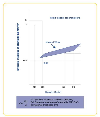
The dynamic stiffness, s', is determined by the test carried out according to the EN 29052-1 standard.
