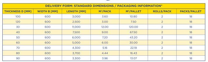
$<sup>^{\</sup>ast}$  All dimensions require minimum order quantities / other dimensions on request. \*\* Under a load of 1,000 Pa.
